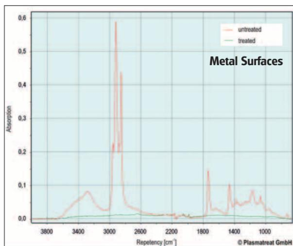
**Fig. 3:** Infrared spectroscopic measurement: During the microfine cleaning of metal surfaces, Openair-Plasma removes all impurities and organic contaminants such as grease, oils and water adhering to the boundary layer.
