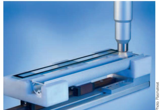
**Fig. 2:** Clean and environmentally friendly: Nowadays Waldmann uses Openair-Plasma instead of solvent-based primers to clean the aluminum housings of the surface-mounted LED machine lights to a microfine level and activate them before bonding.
