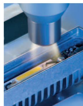
**Fig. 4:** Potential-free plasma pretreatment: Special rotary nozzle heads dissipate the electrical potential in the plasma, making it possible to pretreat even highly sensitive SMD assemblies and other delicate electronic components without damaging them.
