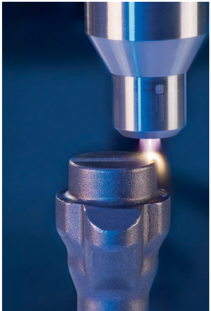
Figure 3 > Openair-Plasma removes all impurities and organic contaminants from metal surfaces.
